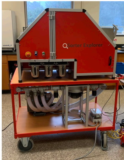
Figure 2.2. QSorter Explorer used to define peanut seed size, oleic acid content, moisture content, splits and seed coat color
