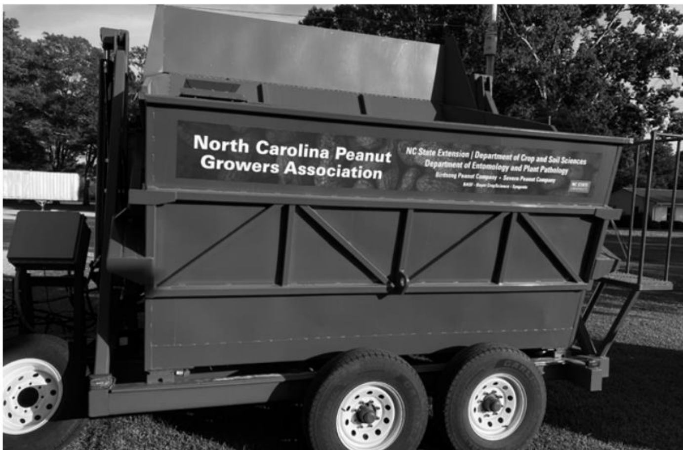
Figure 14-1. A peanut dump cart with a weigh scale was used in large-plot testing. Source: David Jordan
